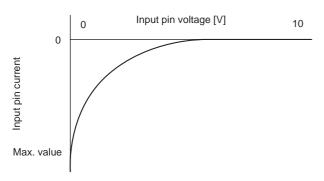
Pull-in current characteristics at the input pin
